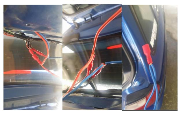
Measure 2 lengths of wire to each lenses from the number plate light, (for me, 1 side was only 20cm long and the other was 40cm) join one end of the wires together & crimp a blade terminal on (pictured below), and then crimp a blade terminal on each other end. Plug the joined end onto the number plate loom, and run each other end to each of the lenses and plug them into the Black wires of the Bulb holder.
